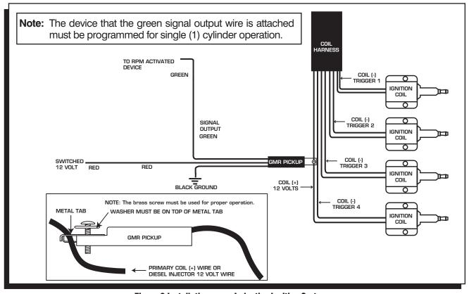
Figure 2 Installation on an Inductive Ignition System.
