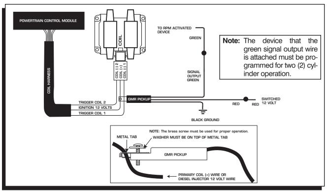
Figure 3 Installation on a Distributorless Coil Pack.
