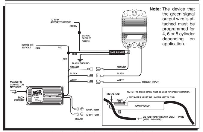
Figure 1 Installation with a Capacitive Discharge Ignition Control.
