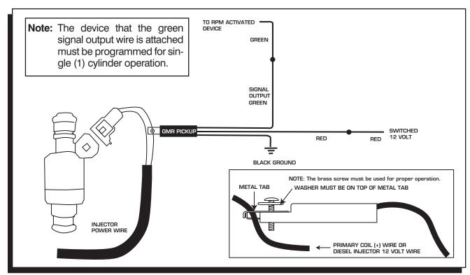
Figure 4 Installation to a Diesel Injector.
